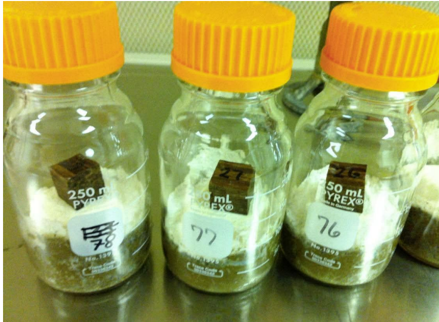
Photograph 10 – Brown Rot Fungi Growth on Soil, but not on Bamboo Samples
