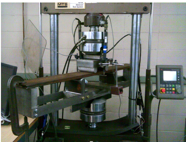
Photograph 2 – Typical Flexural Splice Test Configuration
