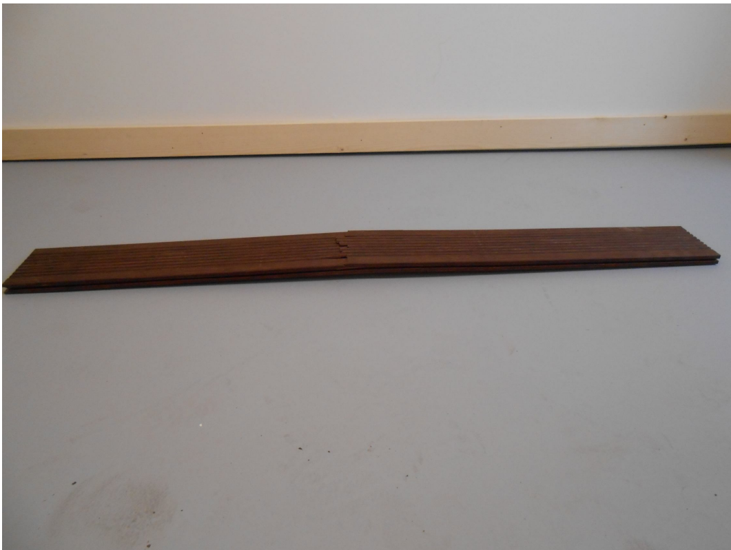
Photograph 9 – Typical Flexural Failure Mode (LS)
