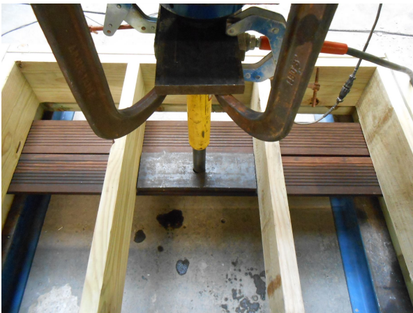
Photograph 6 – Typical Fastener Uplift/Withdrawal Test Configuration
