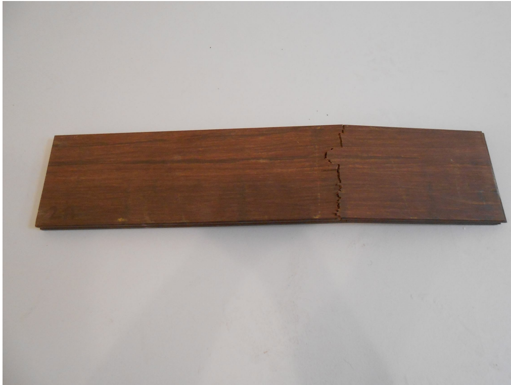
Photograph 8 – Typical Flexural Failure Mode (SC)
