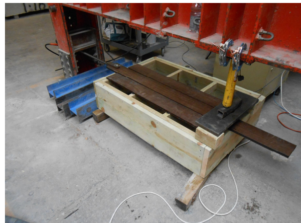
Photograph 7 – Typical Fastener Lateral Load Test Configuration
