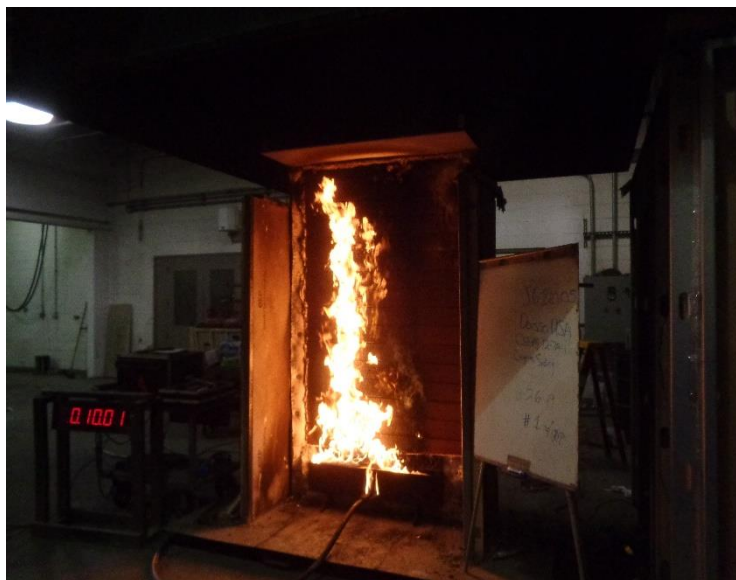
Photo No. 8 Flaming after Burner is Extinguished
