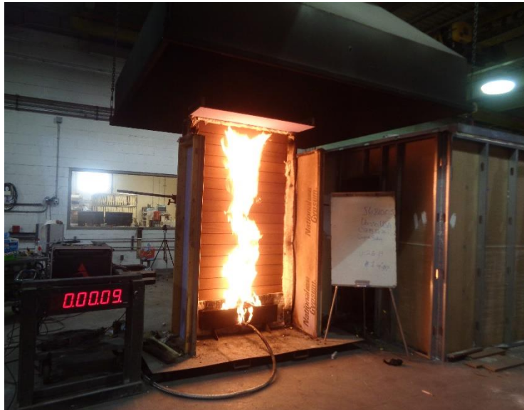
Photo No. 7 Ignition of Burner
