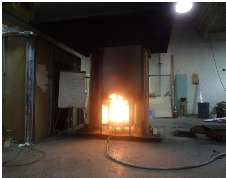
Photo No. 4 Ignition of Burner
