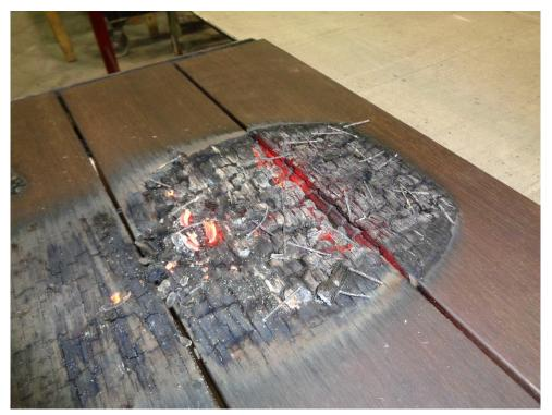
Photo No. 10 Glowing Combustion during Testing
