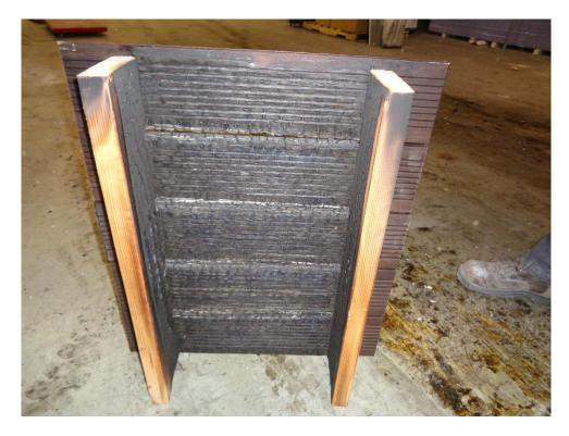
Photo No. 7 Bottom of Underdeck Specimen (Post-test)
