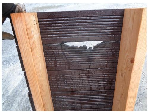
Photo No. 12 Bottom Surface of Burning Brand Deck (Post-test)
