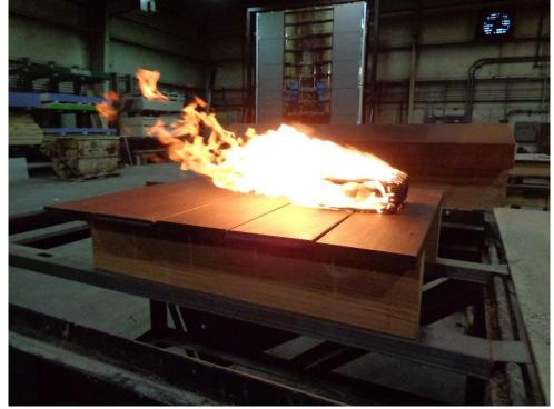
Photo No. 9 Class B Burning Brand Exposure
