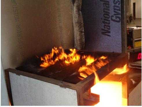
Photo No. 5 Ignition during Underdeck Test
