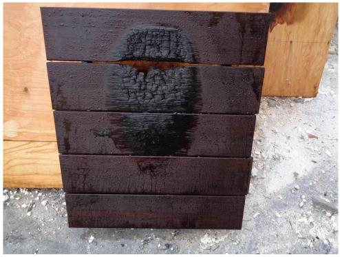
Photo No. 11 Top Surface of Burning Brand Deck (Post-test)
