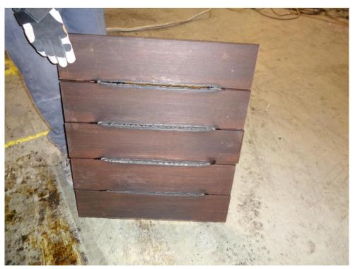
Photo No. 6 Top of Underdeck Specimen (Post-test)
